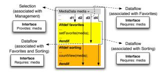
Figure 2. Components and their respective interfaces.
